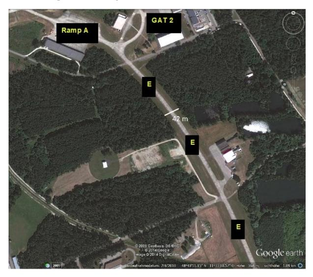
The obstacle wingtip clearance on the taxiway "E" is granted for A/C with a wingspan less than or equal to 15 meters only.
